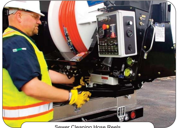
Sewer Cleaning Hose Reels
